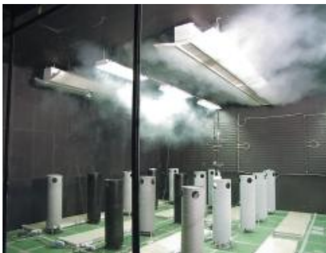
Fig. 20: Air flow pattern and indoor air velocities with one-way discharge chilled beam
