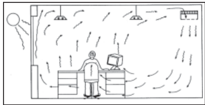
Fig. 10: Chilled beam at or near the corridor wall
