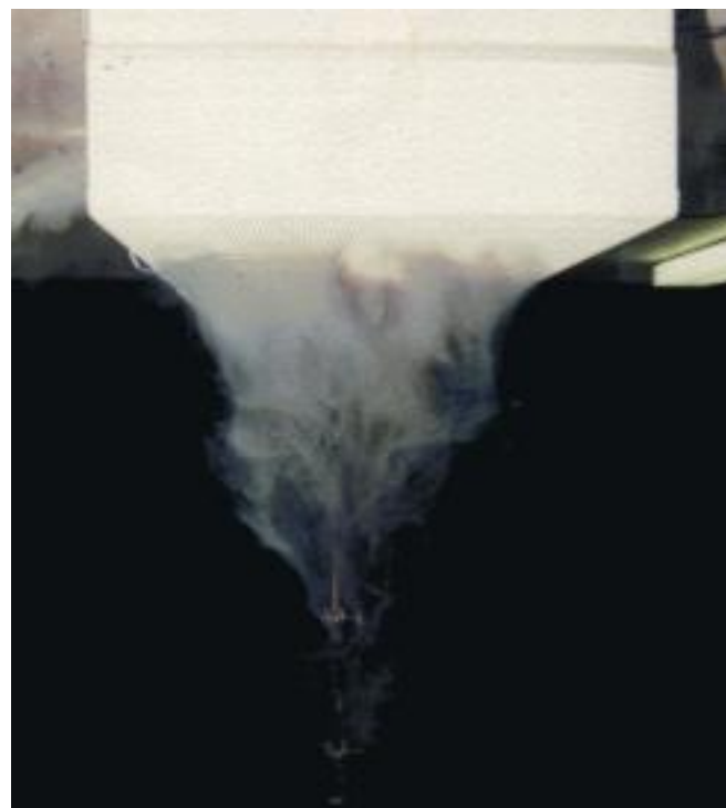
Fig. 7: Indoor air velocities below passive chilled beams in relation to the specific cooling capacity
