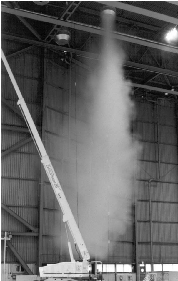
Fig. 5: Penetration depth of supply air jets made visible with a smoke tracer
