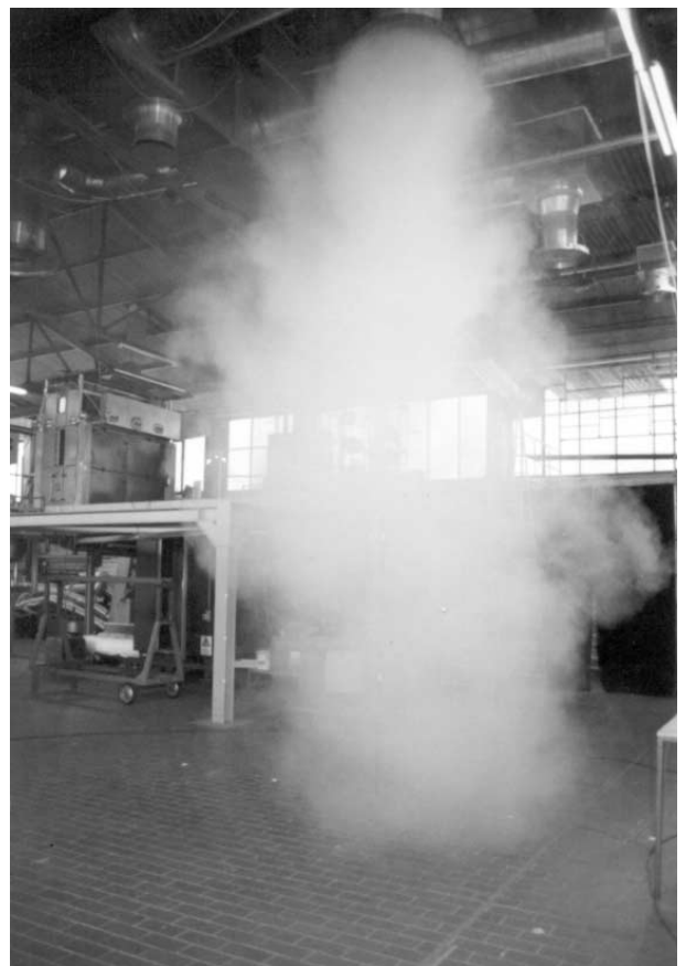
Fig. 8: Vertical discharge from a great height, jet pattern visible using smoke tracer; Above: when cooling, core tube closed, Below: when heating, core tube open.
