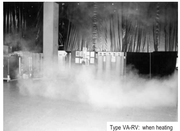
Figure 3: Influence of the adjustment device on discharge flow with corresponding control lever position
