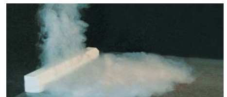
Air jet pattern of Q-SH (when heating)
