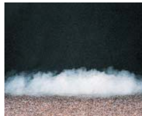
Air jet pattern "displacement flow"
