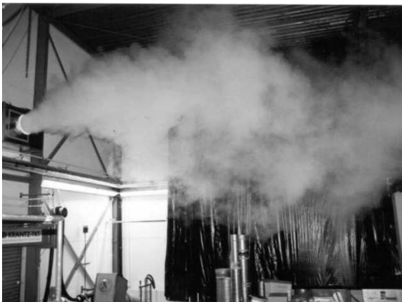
Jet spread when cooling
