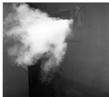
Jet pattern made visible with smoke tracer
